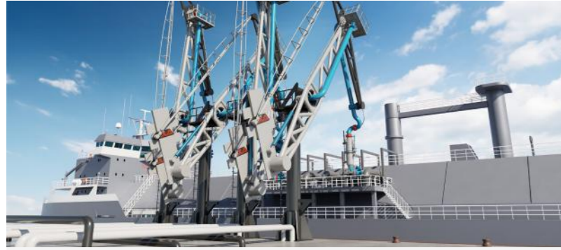
JLA's liquid hydrogen loading arm
